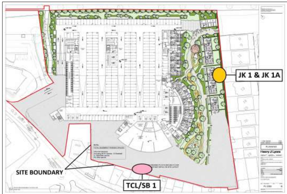
Figure 15 : Location of I.A.P.S. stands in relation to the basement footprint of the development (Source: Henry J. Lyons, Architects)
